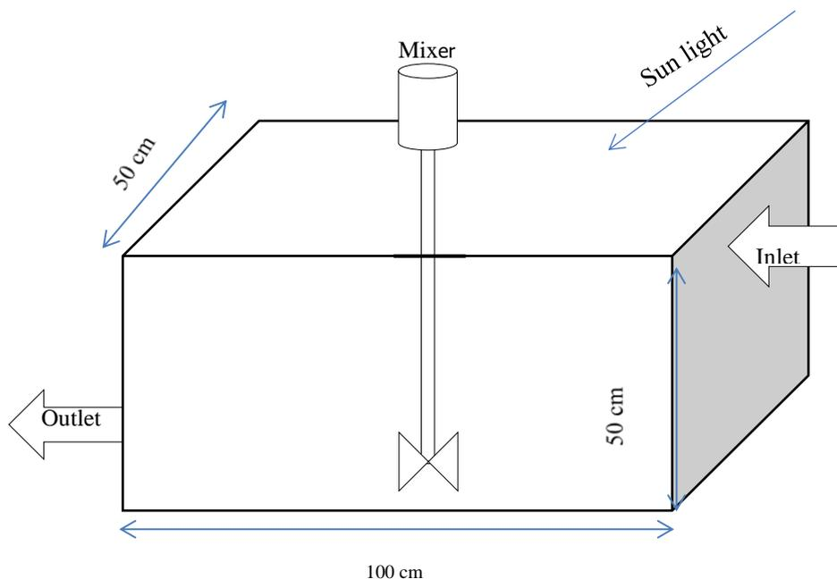
**Fig.1.** Reactor of Fenton Photo method shows the dimensions of it, the reactor made from cleared matter to permit the sunlight to penetrate it reaching to wastewater and the reaction was began
