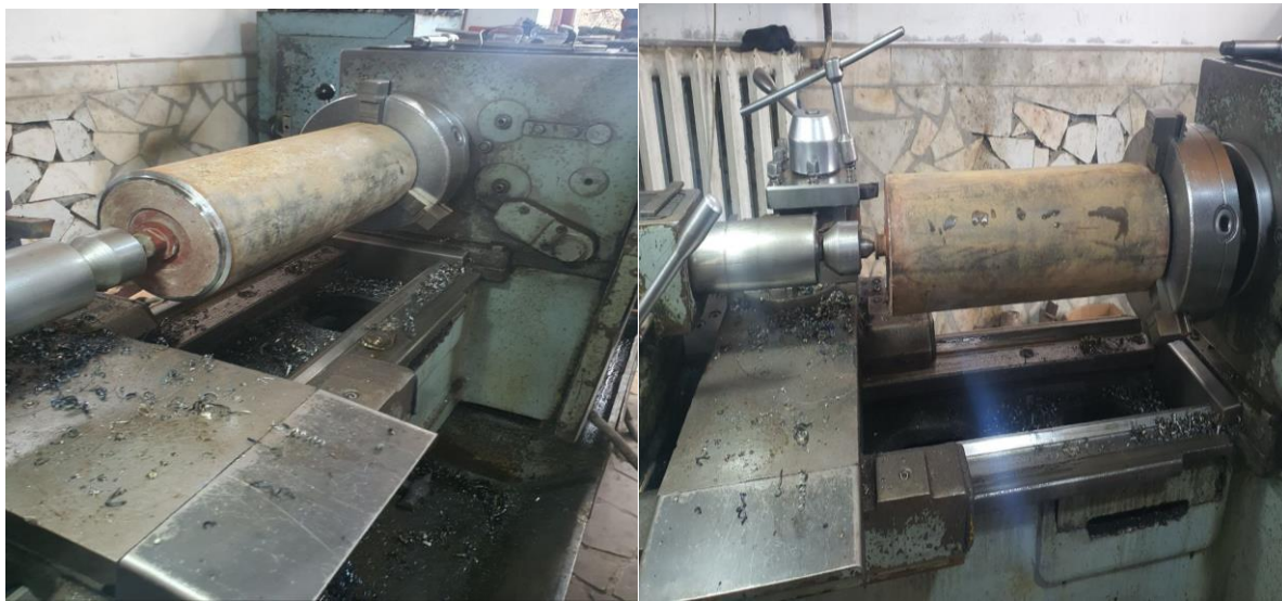
Picture 7. The process of checking the roller axis from center to displacement
