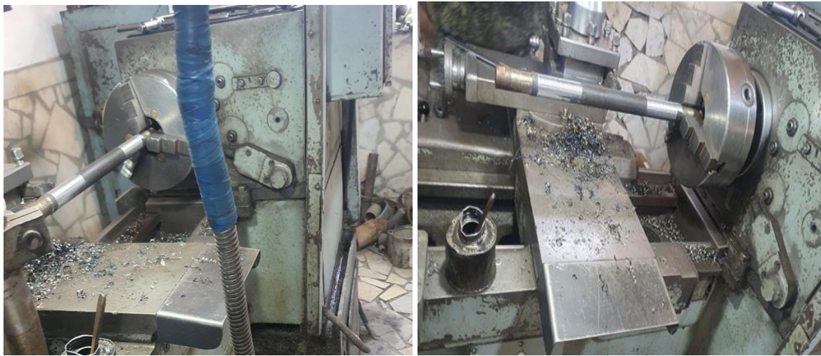
Picture 6. The process of checking the roller axis for flatness
