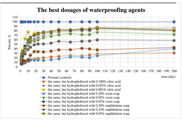
After the cement has been hydrophobized, its ability to absorb moisture from the atmosphere is significantly reduced. The special arrangement of asymmetric polar molecules of hydrophobic surfactants, with hydrocarbon radicals facing outward, promotes the formation of hydrophobic coatings on the cement particles. In this regard, hydrophobized cements usually do not sinter during long-term storage and transportation.
