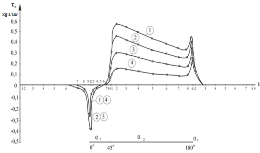
Figure 8. Graph of the Variation of Shear Stresses Along the Coverage of a Five-Layer Belt Under the Combined Influence of Tensile, Bending, and Rotational Forces ( $\sigma=15 \text{ kg/cm}^2$ ,  $E=2500 \text{ kg/cm}^2$ ,  $H=0.19 \text{ cm}$ ,  $D=140 \text{ cm}$ ,  $\delta=0.15 \text{ cm}^2$ ,  $i=5$ ,  $\alpha=1800$ ,  $\beta=450$ ,  $S_o=140 \text{ kg}$ ,  $F_{rp}=0.3$ )
