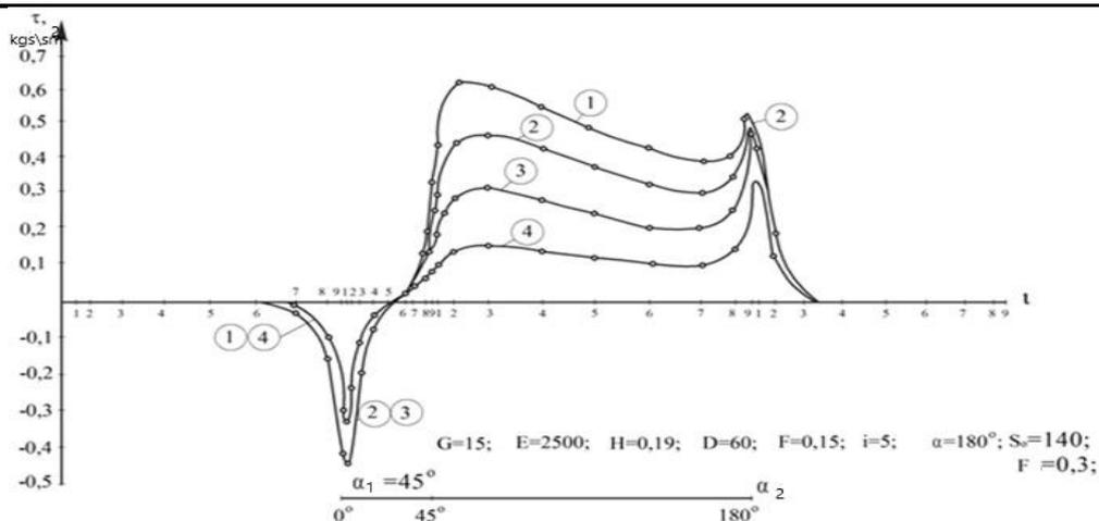
Figure 6. Graph of the Variation of Shear Stresses Along the Coverage of a Five-Layer Conveyor Belt Under the Combined Influence of Tensile, Bending, and Tension Forces ( $G=15 \text{ kg/cm}^2, E=2500 \text{ kg/cm}^2, H=0.19 \text{ cm}, D=60 \text{ cm}, \delta=0.15 \text{ cm}^2, i=5, \alpha=180^\circ, \beta=45^\circ, S_o=140 \text{ kg}, F_{Tp}=0.3$ )
