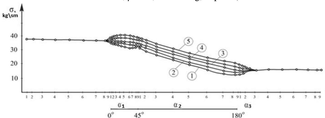
Figure 4. Graph of the Variation of Tensile Stresses Along the Coverage of a Five-Layer Conveyor Belt ( $\sigma=15 \text{ kg/cm}^2$ ,  $E=2500 \text{ kg/cm}^2$ ,  $H=0.19 \text{ cm}$ ,  $D=60 \text{ cm}$ ,  $\delta=0.15 \text{ cm}^2$ ,  $i=5$ ,  $\alpha=1800$ ,  $\beta=450$ ,  $S_o=140 \text{ kg}$ ,  $F_{Tp}=0.3$ )
