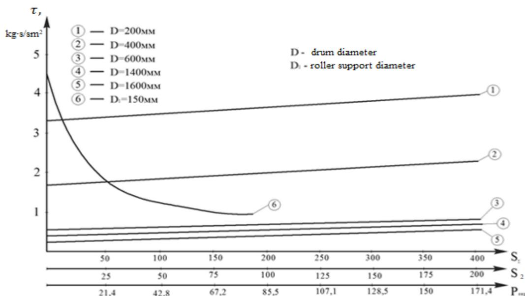
Figure 13. Nomogram of the Relationship Between Drum Diameter, Initial Belt Tension, and Tensioning Force.
