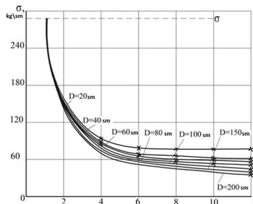
**Figure 2.** Graph of the stresses in the layers of a nylon-based conveyor belt, related to the number of layers under tension, bending, and tensile forces.
