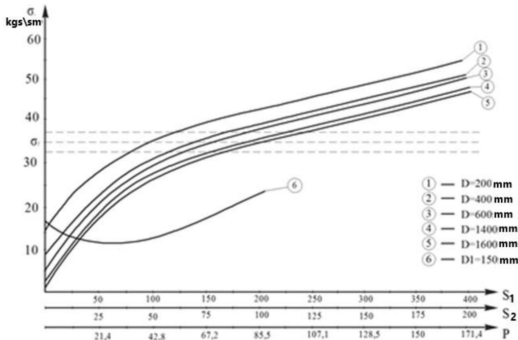
Figure 12. Nomogram of the Relationship Between Drum Diameters, Initial Belt Tension, and Tensioning Force.
