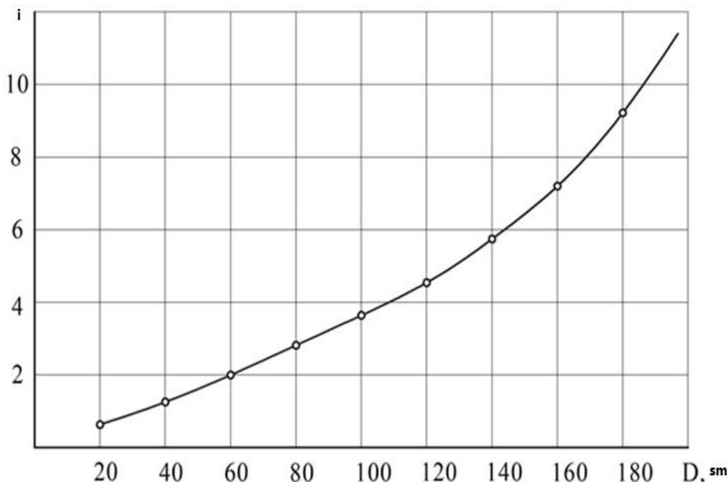
Figure 11. Graph of the Relationship Between the Number of Belt Layers and Drum Diameter
