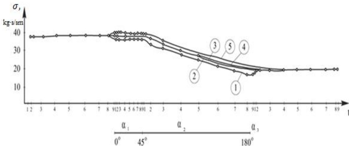
Figure 9. Graph of the Variation of Tension Stresses Along the Coverage of a Five-Layer Conveyor Belt ( $\sigma=15 \text{ kg/cm}^2$ ,  $E=2500 \text{ kg/cm}^2$ ,  $H=0.19 \text{ cm}$ ,  $D=160 \text{ cm}$ ,  $\delta=0.15 \text{ cm}^2$ ,  $i=5$ ,  $\alpha=1800$ ,  $\beta=450$ ,  $S_o=140 \text{ kg}$ ,  $F_{rp}=0.3$ )
