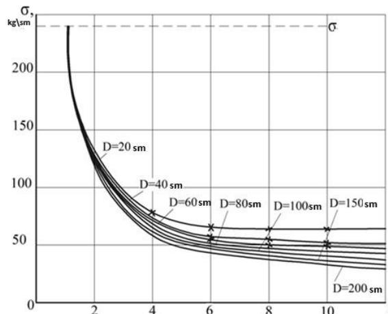
**Figure 1.** Graph of the stresses in the layers of a nylon-based conveyor belt, related to the number of layers under tension, bending, and tensile forces.
