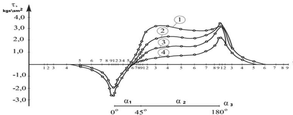
Figure 5. Graph of the Variation of Shear Stresses Along the Coverage of a Five-Layer Conveyor Belt Under the Combined Influence of Tensile, Bending, and Tension Forces ( $\sigma=15 \text{ kg/cm}^2$ ,  $E=2500 \text{ kg/cm}^2$ ,  $H=0.19 \text{ cm}$ ,  $D=20 \text{ cm}$ ,  $\delta=0.15 \text{ cm}^2$ ,  $i=5$ ,  $\alpha=1800$ ,  $\beta=450$ ,  $S_o=140 \text{ kg}$ ,  $F_{Tp}=0.3$ )
