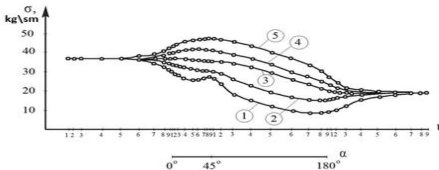
Figure 3. Graph of the Variation of Tensile Stresses Along the Coverage of a Five-Layer Conveyor Belt ( $\sigma=15 \text{ kg/cm}^2$ ,  $E=2500 \text{ kg/cm}^2$ ,  $H=0.19 \text{ cm}$ ,  $D=20 \text{ cm}$ ,  $\delta=0.15 \text{ cm}^2$ ,  $i=5$ ,  $\alpha=1800$ ,  $\beta=450$ ,  $S_o=140 \text{ kg}$ ,  $F_{Tp}=0.3$ )
