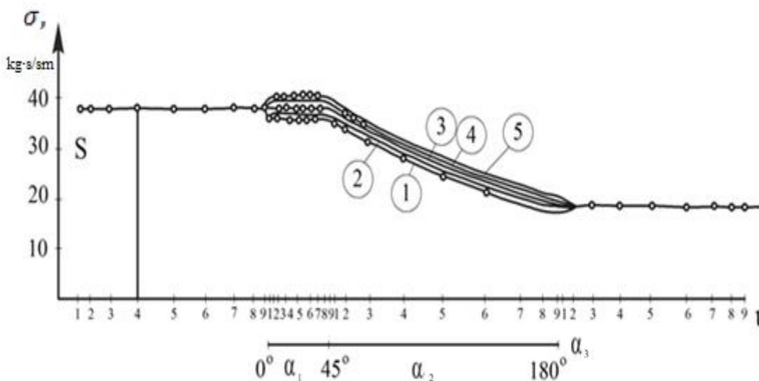
Figure 10. Graph of the Variation of Tension Stresses Along the Coverage of a Five-Layer Conveyor Belt ( $\sigma=15 \text{ kg/cm}^2$ ,  $E=2500 \text{ kg/cm}^2$ ,  $H=0.19 \text{ cm}$ ,  $D=140 \text{ cm}$ ,  $\delta=0.15 \text{ cm}^2$ ,  $i=5$ ,  $\alpha=180$ ,  $\beta=450$ ,  $S_0=140 \text{ kg}$ ,  $F_{Tp}=0.3$ )
