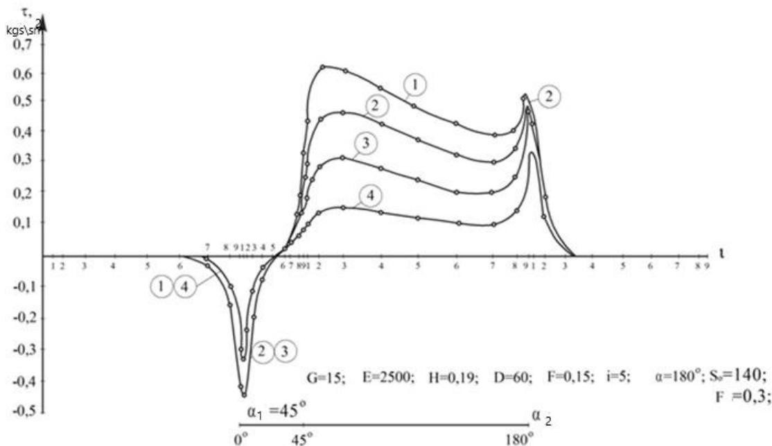
Figure 7. Graph of the Variation of Shear Stresses Along the Coverage of a Five-Layer Belt Under the Combined Influence of Tensile, Bending, and Rotational Forces ( $G=15 \text{ kg/cm}^2, E=2500 \text{ kg/cm}^2, H=0.19 \text{ cm}, D=160 \text{ cm}, \delta=0.15 \text{ cm}^2, i=5, \alpha=180^\circ, \beta=45^\circ, S_o=140 \text{ kg}, F_{Tp}=0.3$ )
