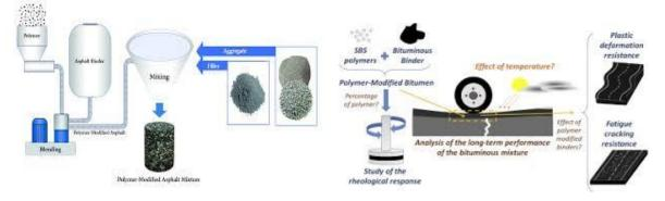
The preparation of reinforced polymer-bitumen compositions involves several key technologies to enhance the performance and durability of bitumen used in road construction.
