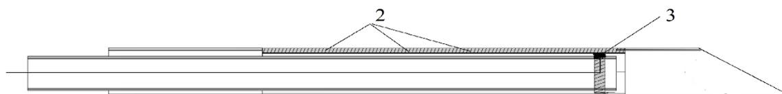
c) sectional side view, 2 - insulated strips or wires in dielectric plate 3 - dielectric rod protrusion with contact surface
