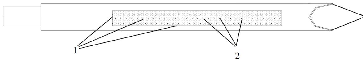
b) 1 – dielectric plate, 2 –insulated metal wires
