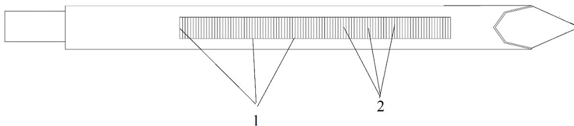
a) 1 – dielectric plate, fixed in the longitudinal cutout of needle electrode, 2 –insulated metal strips
