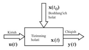
1-picture. Data entry and output parameters of the system are given.
