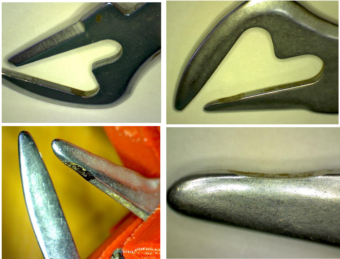
Drawing. 1. Wear of the internal contact surfaces of the baton teeth
