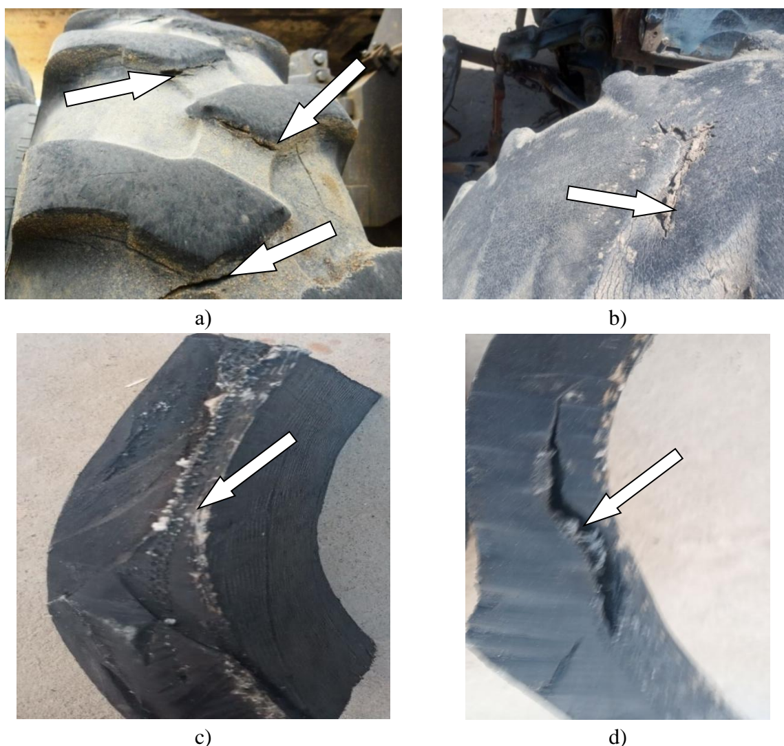
Fig. 1. Defects and damage to pneumatic tires.
