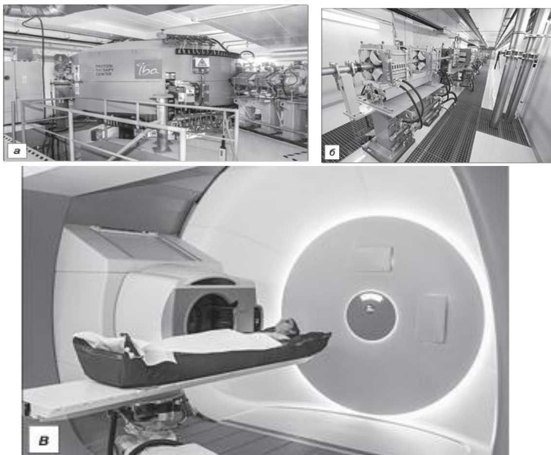
Fig. Photographs of the cyclotron (a), the proton beam transport system (b), and the rotating gantry irradiation unit with a robotic table (c) in the "Oncology Proton Therapy Center".
