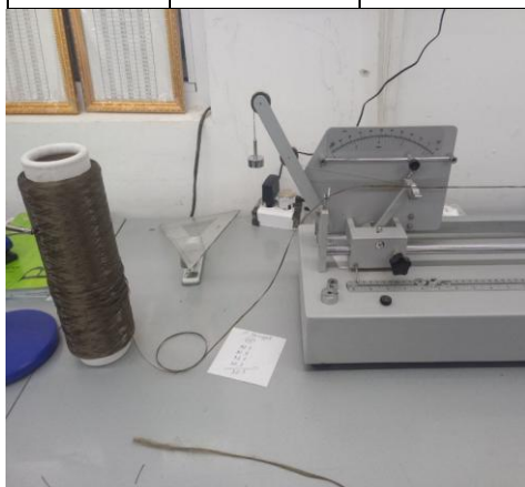
Fig. 2. Machine for determining the number of twists in basalt fiber
