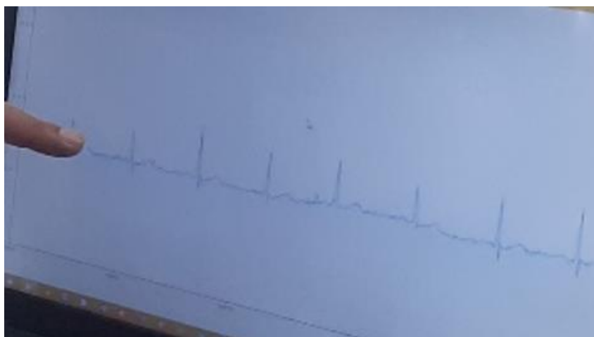
2.15-rasm. EkG image taken using the AD8232 EKG module. time in the ordinary-amplitude, obsissada.
