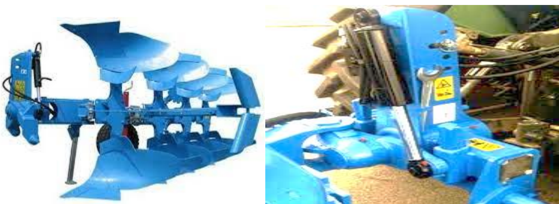
Fig.1. It is usual wheeling mechanism of floating ploughs – hydraulic mechanism
