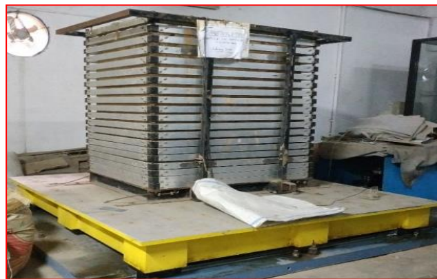
Figure 1. Seismic analysis of the model embankment
