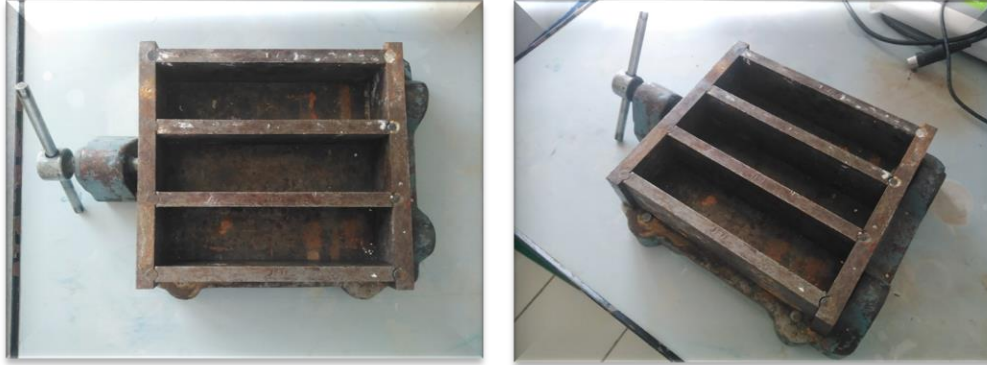
Figure 1. The dimensions are 4x4x16 cm has been mould appearance
