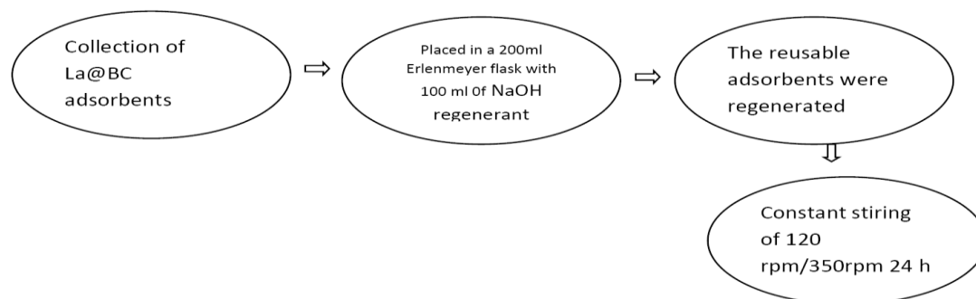
Fig-1: Flow chart about phosphate removal by Batch process using La@BC adsorbents
