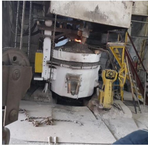
Figure 1. Melting process of 35XГCЛ steel alloy in a 500 kg electric arc furnace in the foundry mechanics workshop of "UzMetkombinat" JSC [9].
