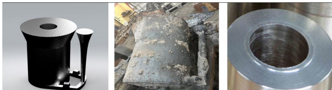
Figure 3. 35XГCJI low – alloy steel melt – cast shaft detail without defects
