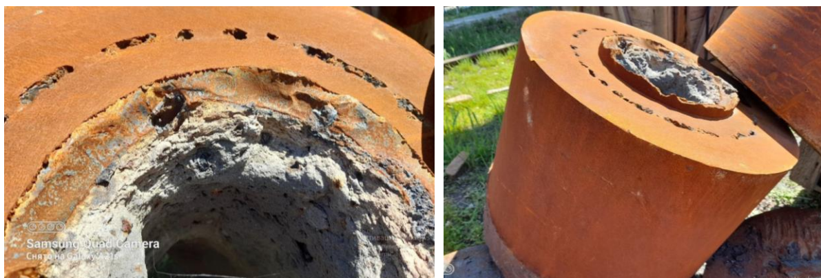
Figure 2. Defects of cast shafts are shown
