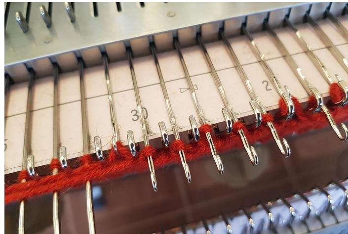
Figure 2. Needle structure of a flat needle knitting machine
