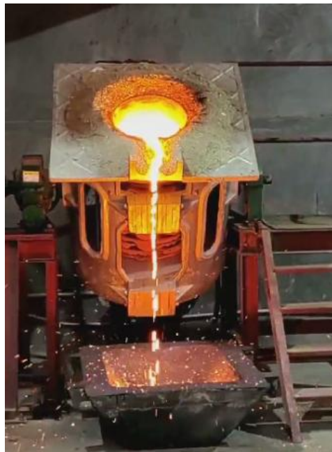
1 – fig. The process of melting metal in an induction furnace
