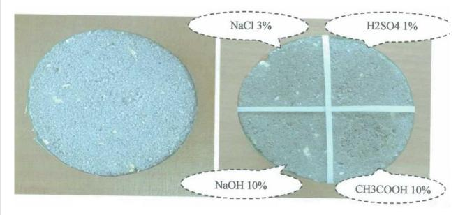
After treating the surface of sample No. 2 (see Figure 2), which contains sulfur binder without heat treatment, damage is also noticeable in the sector exposed to acetic acid and other reagents, but there is less damage than when processing conventional concrete.
