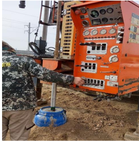
Figure 4. The proposed construction is an experimental test of an improved three-ball dolota and diamond-toothed coronac.
