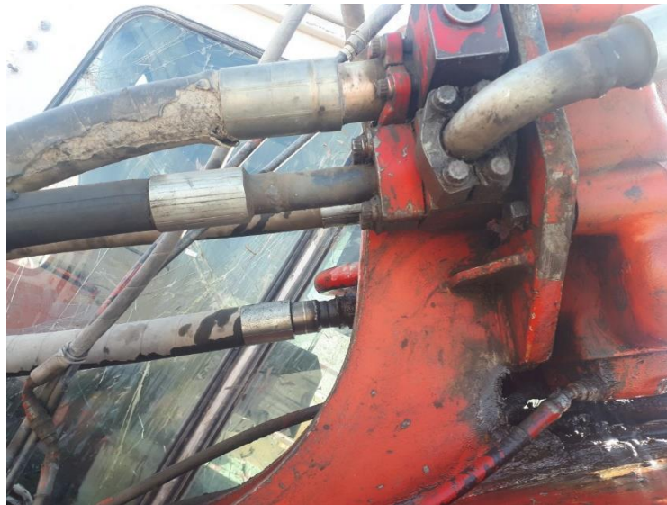
Figure 1. The state of connection of the skirts in the working organs of the excavator of the RH-40E brand
