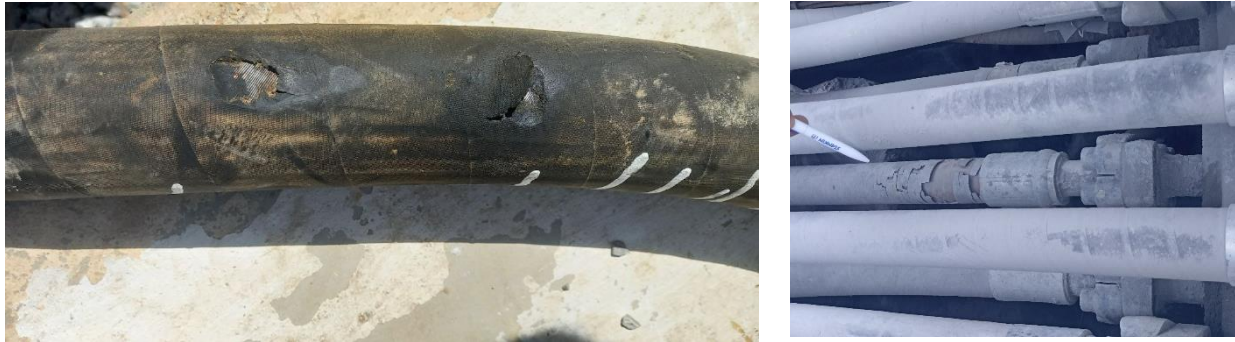
Figure 2. The condition of the rukavs with the loss of reliable working capacity of their external rubber.
