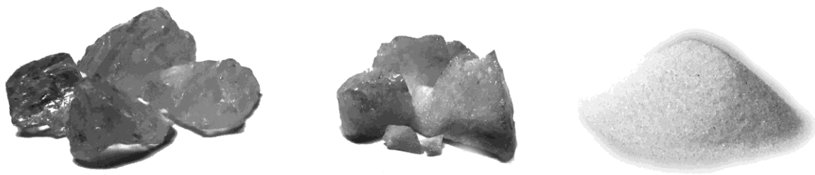
Fig. 2. Quartz crystals (a), quartz after fritting (b), ground quartz (c)
