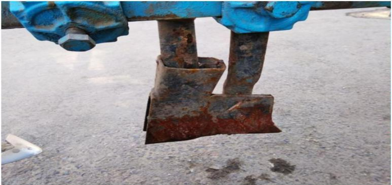
Fig. 5. Shows the corrosion damage to the parts of a working cultivator.
