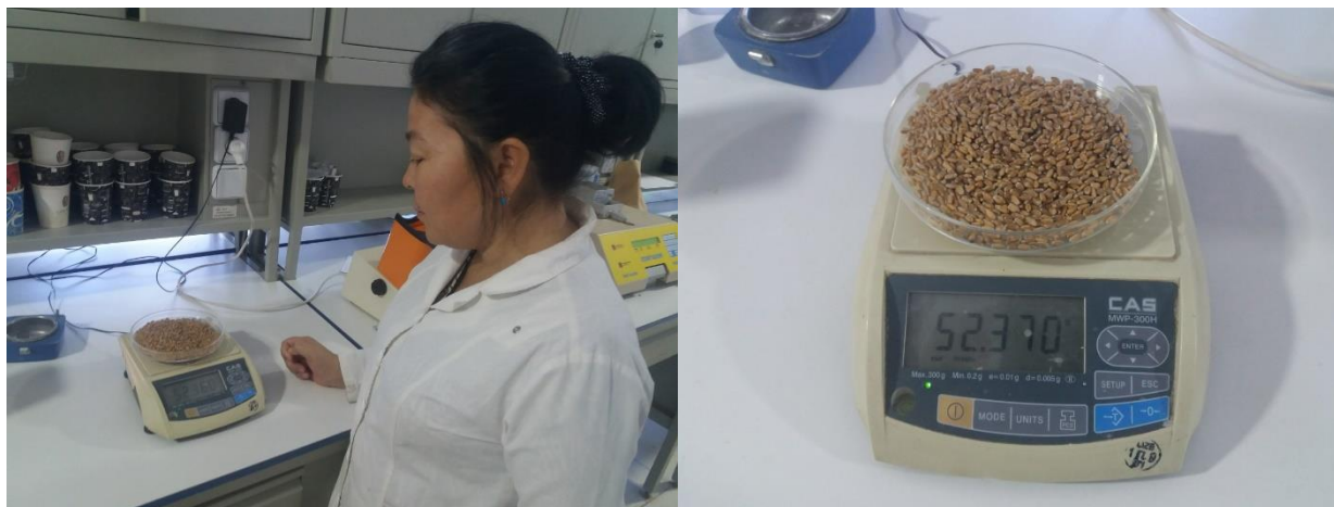
1-picture «The process of determining the mass of 1000 grains of the «Turon» variety.
