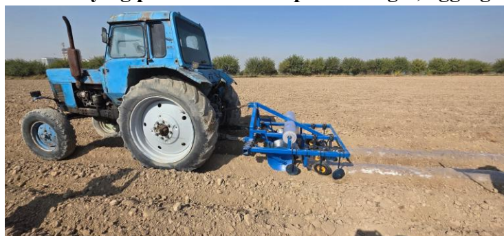
Figure 3. Machine for laying plastic film on potato-planted ridges.
