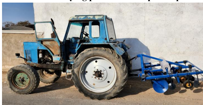
Figure 2. A machine for laying plastic film over potato ridges, aggregated with a tractor.
