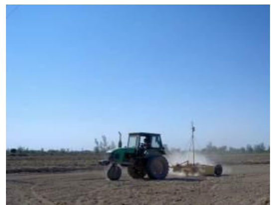
Figure 3. Topographic surveying and land leveling using laser equipment.
