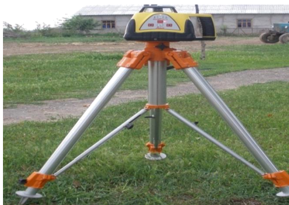
Figure 3. Topographic surveying and land leveling using laser equipment.
